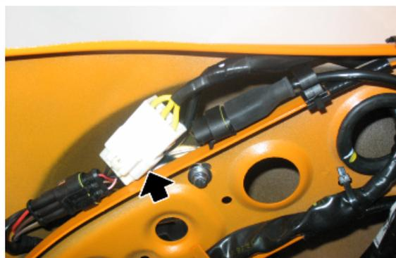
**2. Voltage regulator** - Remove the front central cover to reach it.
