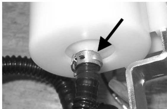
Separate the lower part of the pump mounting as shown in the picture.
