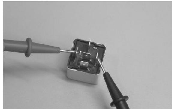
Check the presence of fixed voltage between the Red-White cable of the relay base and ground.
