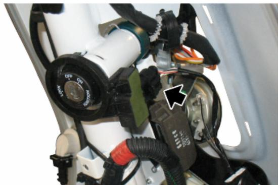
Remove the protective base from the connector.
