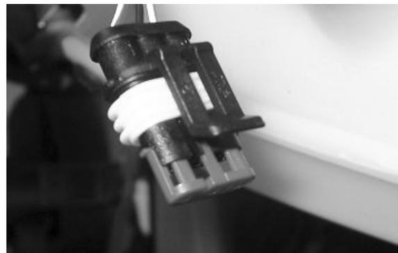
With the ignition switch at ON check there is battery voltage between the Orange-Blue and Black cables.
