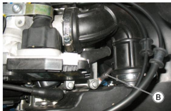
On the left side of the chassis, under the footrest, there is the chassis-engine ground lead "C".
