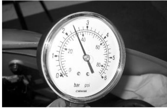
With the battery voltage > 12 V, check the pump flow rate by disconnecting from the injector the pipe equipped with the pressure gauge of the appropriate tool. Make a graded burette available with a flow rate of approximately 1 L. Rotate the pump using the active diagnosis of the palm top computer. Using a pair of long flat needle-nose pliers, choke the fuel pipe making the pressure stabilise at approx. 2.5 bar. Check that within 15 seconds the pump has a flow rate of approx. 110 cm<sup>3</sup>.
