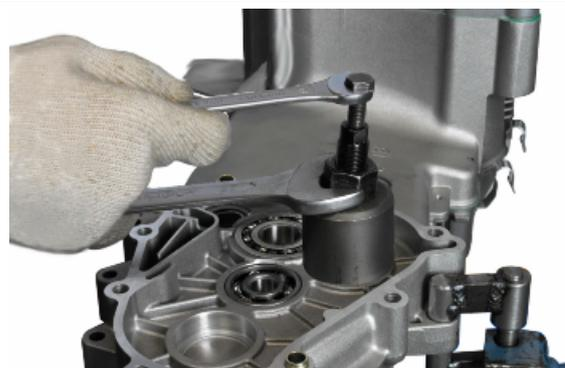
**Removing the Wheel axle bearing**
