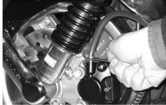
If necessary, bleeding can be done using a special vacuum pump
