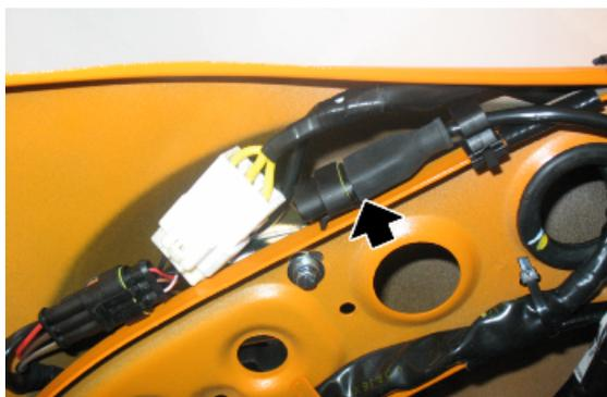
**31 - 32. Engine temperature sensor - fuel injector** - Remove the helmet compartment to reach it.
