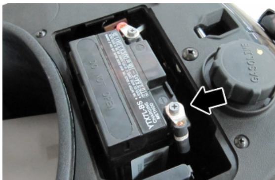
**4. Starter remote control** - Remove the battery to reach it.
