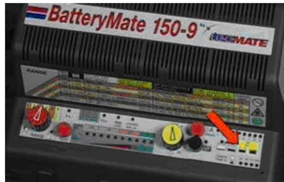
h - Disconnect the clamps from the battery and check the voltage, if voltages are detected of less than 12.8 V, proceed with a new recharge of the battery starting from point c of the recharge procedure of **the new battery**, otherwise go to point i
