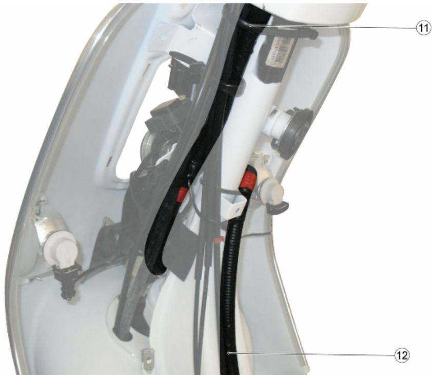
**11.** Connecting branch controls on the driver and the front headlights
