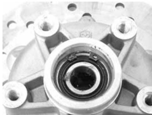
Extract the ball bearing using the specific tool
