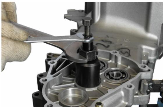
**Removing the wheel axle bearings**
