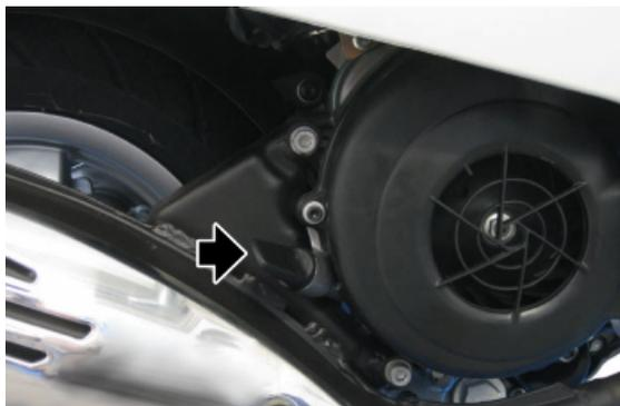
Make sure the pre-filter and drainage plug O-rings are in good conditions.
