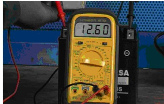
i - The battery is now completely activated, disconnect the battery charger from the fuel supply grid, disconnect the clamps from the battery and proceed to fitting the battery on the vehicle.
