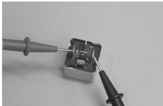
Check the presence of fixed voltage between the Red-White cable of the relay base and ground. Otherwise, check the continuity of the Red-White cable between the fuse-box (No. 6, 10 A) and the relay base.
